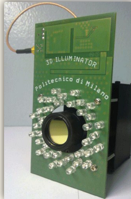
MiSPiA illuminator for the indirect iTOF laboratory tests
